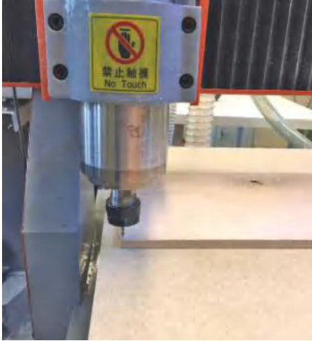
▲ Pic.13 Positioning the router cutter on the top of the left-hand corner of the work
